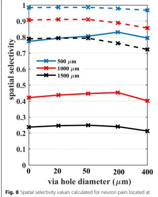
Fig. 8 Spatial selectivity values calculated for neuron pairs located at different depths (500, 1000, and 1500  $\mu$ m) and for different sizes of the via holes. The distance between Neuron A and B is either 707  $\mu$ m (solid lines) or 2121  $\mu$ m (dash lines) as shown in Fig. 2. In all cases, the signals were recorded at the contact that is aligned with Neuron A
