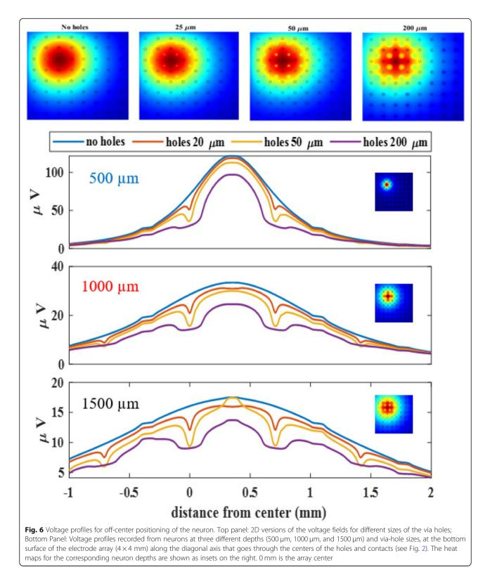
the current flowing through the holes would increase the rate of decline in the extracellular voltage in the vertical direction. The simulations of the current study provided some general guidelines on how the signal amplitudes vary with the hole size. The impact slightly depends on the depth of the targeted neurons for recording. As a practical guideline, 200  $\mu$ m holes will cause about 25% reduction in the recorded signals from the rat
